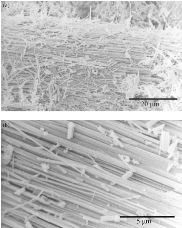
**Figure 1.** SEM images of (a) a bunch of (Na-intercalated) manganese oxide nanowires formed among randomly generated nanowires and (b) a close view of individual nanowires.
