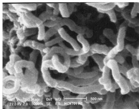
**Figure 1.** SEM image of the carbon nanotubes grown by means of CCVD using BaCl<sub>2</sub>/CaCl<sub>2</sub> catalyst support.
