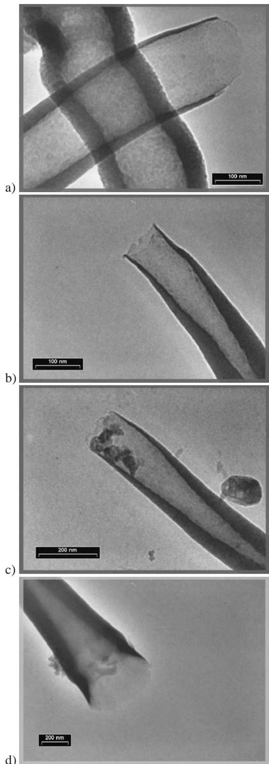
**Figure 2.** TEM images of individual carbon nanotubes.
