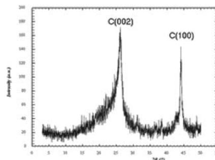
**Figure 3.** XRD Pattern of the cone-like carbon nanotubes.
